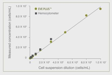
Measuring from the EVE™ PLUS extends further the high concentration range than hemocytometer readings
