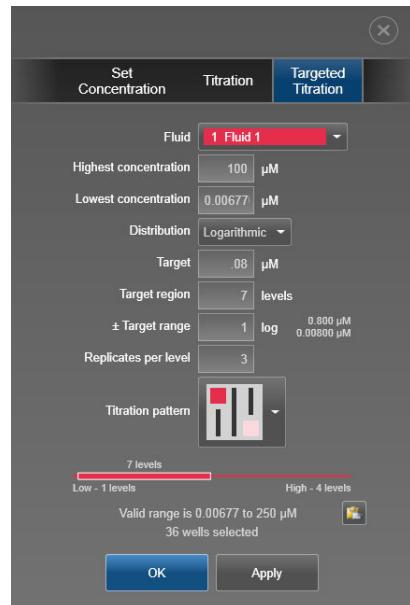
**Figure 4** The Targeted Titration window enables users to set up a titration with a specified number of doses around a certain concentration. This allows a high number of doses to be created around the  $\text{IC}_{50}/\text{EC}_{50}$  value.
