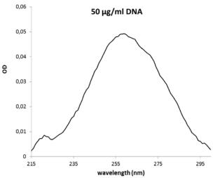
Figure 3: DNA spectrum (50  $\mu$ g/ml sample) after blank reduction measured in the NanoQuant Plate using 2  $\mu$ l sample volume.
