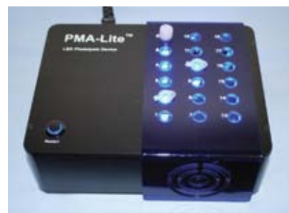
Figure 3. PMA-Lite™ LED Photolysis Device.
