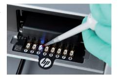
**Loading guide** identifies the correct pipetting location, walking users through the loading process for faster, simpler, more accurate operation.
