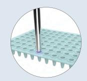
Single well detector-based (non-fiber optic) systems must move 96 times to read each channel.
