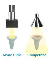
Single illumination light sources can deliver light both in and out of the wells, resulting in higher background, and less light hitting the sample. Azure Cielo uses fiber optics to directly deliver light to each indivdual well.
