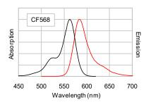
Figure 1. Absorption and emission spectra of CF568 goat anti-mouse conjugate in PBS.
