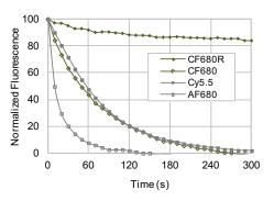
Figure 3. Photostability of far red dye conjugates. Jurkat cells were stained with mouse anti-CD3 followed by the indicated goat anti-mouse IgG conjugates. Cells were continuously exposed to mercury arc lamp excitation with a Cy5 filter set. Images were captured every 10 seconds for 5 minutes and fluorescence intensity was normalized to time 0.
