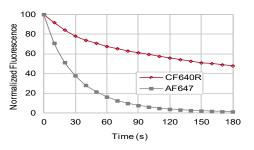
Figure 3. Photostability comparison between CF640R and Alexa Fluor 647 (AF647). HeLa cells were stained with anti-tubulin antibody conjugates of each dye. Cells were continuously illuminated by a mercury arc lamp microscope and sequential images were captured at 0, 1, and 3 minutes. Mean fluorescence was normalized to time 0.
