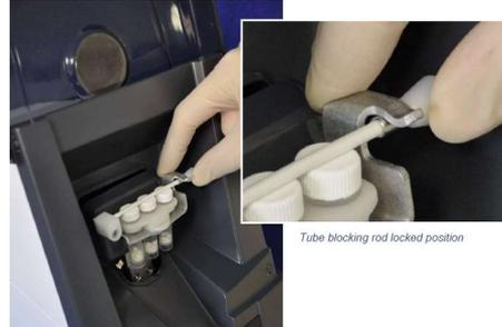
Tube blocking rod locked position
